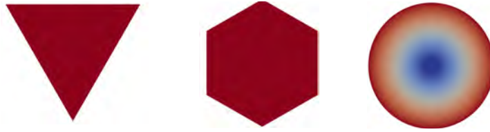
Figure 10: Quadratic VTK_BEZIER_TRIANGLE cell that represents exactly a full disk (this is actually the minimal parameterization of an exact full disk). Nonlinear subdivision level 0, 1 and 5.
