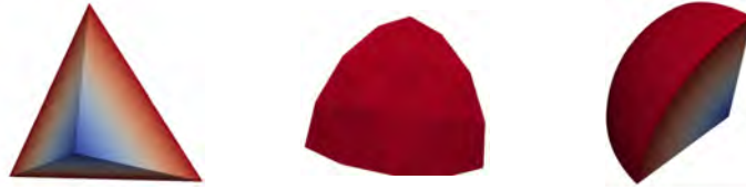
Figure 14: Quartic VTK_BEZIER_TETRAHEDRON cell that represents exactly a solid sphere octant. Nonlinear subdivision level 0, 1 and 5.
