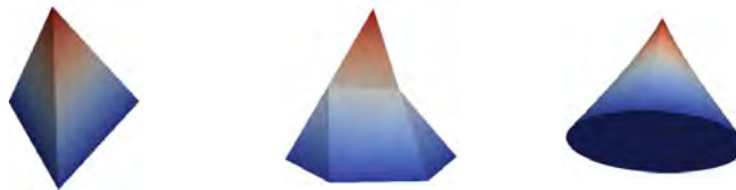
Figure 13: Quadratic VTK_BEZIER_TETRAHEDRON cell that represents a kind of cone. Nonlinear subdivision level 0, 1 and 5.
