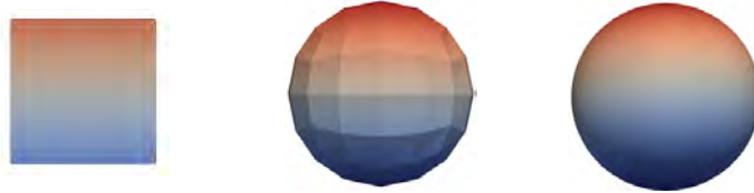
Figure 15: Quartic VTK_BEZIER_HEXAHEDRON cell that represents exactly a sphere. Nonlinear subdivision level 0, 1 and 5.
